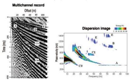
The dispersion curve is an interpretation of the different modes or harmonics of the surface wave as it propagates through a given media. The Vs30 parameter is calculated by taking a weighted average
